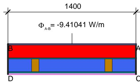
$$U_{eq A-B} = \frac{\Phi}{\Delta T \cdot b} = \frac{9.410}{30.000 \cdot 1.400} = 0.224 \text{ W}/(\text{m}^2 \cdot \text{K})$$
