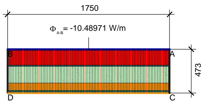
$$U_{\text{eq A-B}} = \frac{\Phi}{\Delta T \cdot b} = \frac{10.490}{30.000 \cdot 1.750} = 0.200 \text{ W}/(\text{m}^2 \cdot \text{K})$$
