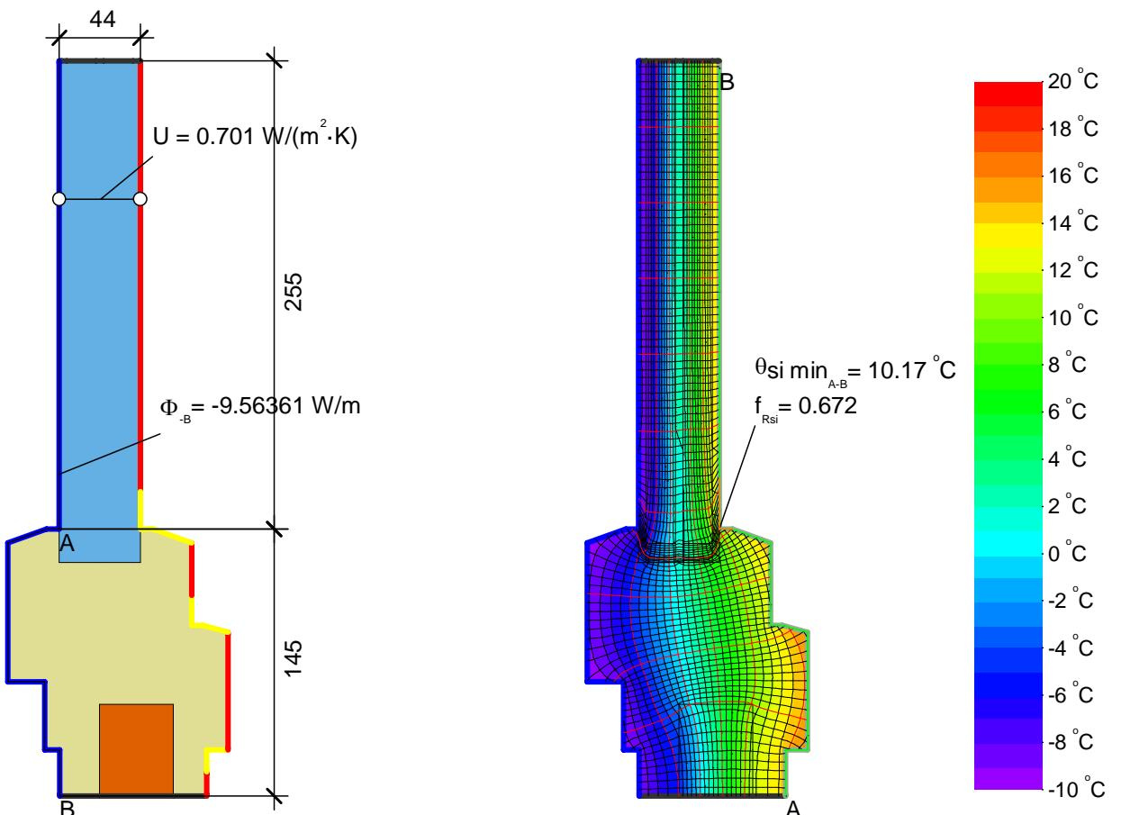
$$U_{f,A,B} = \frac{\frac{\Phi}{\Delta T} - U_p \cdot b_p}{b_f} = \frac{\frac{9.564}{30.000} - 0.701 \cdot 0.255}{0.145} = 0.966 \text{ W}/(\text{m}^2 \cdot \text{K})$$
