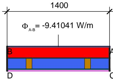
$$U_{eq\ A-B} = \frac{\Phi}{\Delta T \cdot b} = \frac{9.410}{30.000 \cdot 1.400} = 0.224 \text{ W/(m}^2\text{·K)}$$
