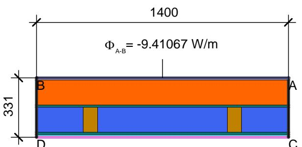
$$U_{eq A-B} = \frac{\Phi}{\Delta T \cdot b} = \frac{9.411}{30.000 \cdot 1.400} = 0.224 \text{ W}/(\text{m}^2 \cdot \text{K})$$
