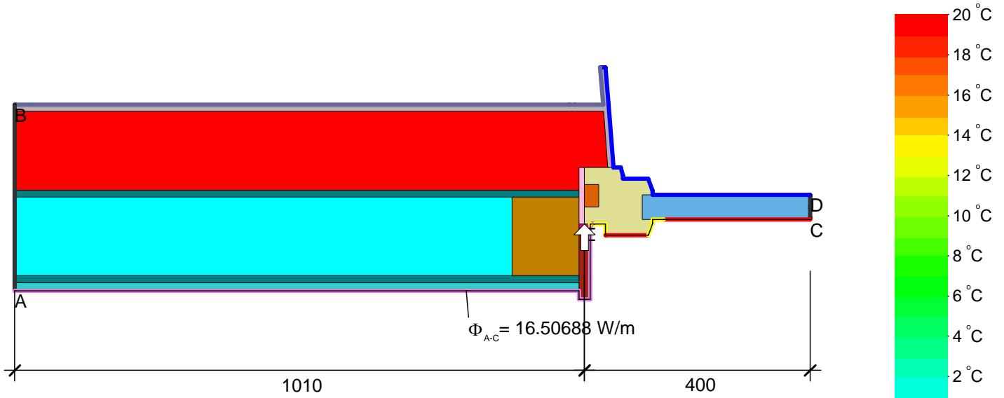
$$\psi_{A-E-C,-} = \frac{\Phi}{\Delta T} - U_1 \cdot b_1 - \frac{\Phi_2}{\Delta T} = \frac{16.507}{30.000} - 0.224 \cdot 1.010 - \frac{9.454}{30.000} = 0.009 \text{ W/(m}\cdot\text{K)}$$
