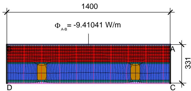
$$U_{eq\ A-B} = \frac{\Phi}{\Delta T \cdot b} = \frac{9.410}{30.000 \cdot 1.400} = 0.224 \text{ W/(m}^2\text{·K)}$$
