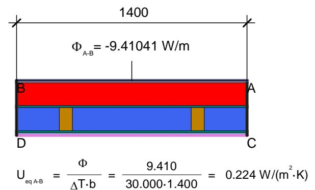
$$U_{eq A-B} = \frac{\Phi}{\Delta T \cdot b} = \frac{9.410}{30.000 \cdot 1.400} = 0.224 \text{ W}/(\text{m}^2 \cdot \text{K})$$
