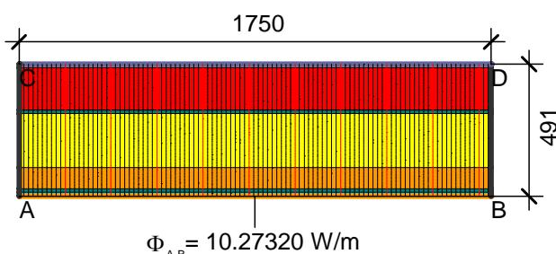
$$U_{\text{eq A-B}} = \frac{\Phi}{\Delta T \cdot b} = \frac{10.273}{30.000 \cdot 1.750} = 0.196 \text{ W}/(\text{m}^2 \cdot \text{K})$$
