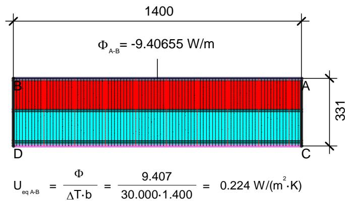
$$U_{eq\ A-B} = \frac{\Phi}{\Delta T \cdot b} = \frac{9.407}{30.000 \cdot 1.400} = 0.224 \text{ W/(m}^2\text{·K)}$$
