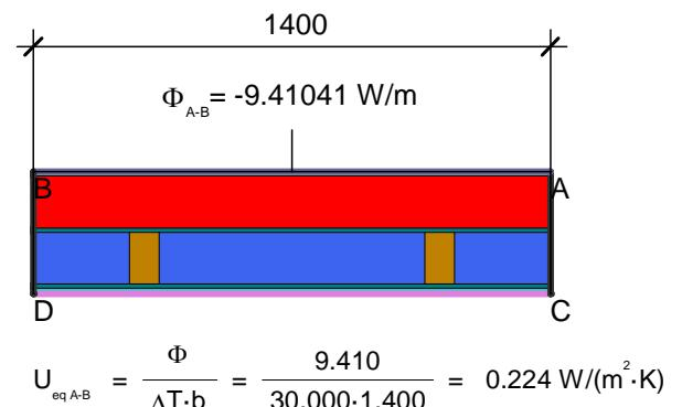
$$U_{eq A-B} = \frac{\Phi}{\Delta T \cdot b} = \frac{9.410}{30.000 \cdot 1.400} = 0.224 \text{ W/(m}^2\cdot\text{K)}$$
