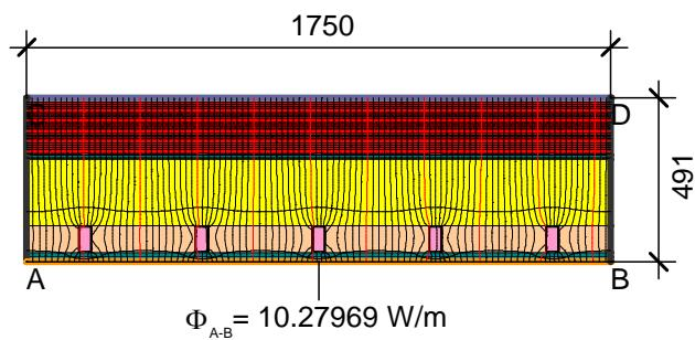
$$U_{\text{eq A-B}} = \frac{\Phi}{\Delta T \cdot b} = \frac{10.280}{30.000 \cdot 1.750} = 0.196 \text{ W}/(\text{m}^2 \cdot \text{K})$$
