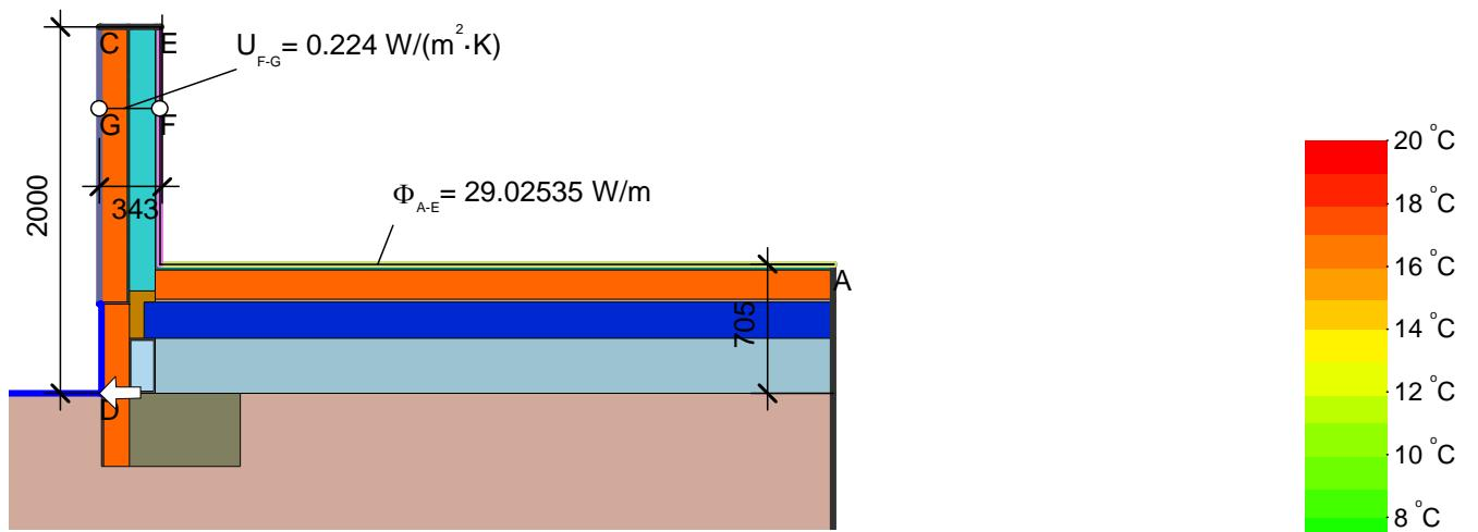
$$\psi_{A-D-E, \dots} = \frac{\Phi}{\Delta T} - \frac{\Phi_1}{\Delta T} - U_2 \cdot b_2 = \frac{29.025}{30.000} - \frac{18.611}{30.000} - 0.224 \cdot 2.000 = -0.101 \text{ W}/(\text{m} \cdot \text{K})$$
