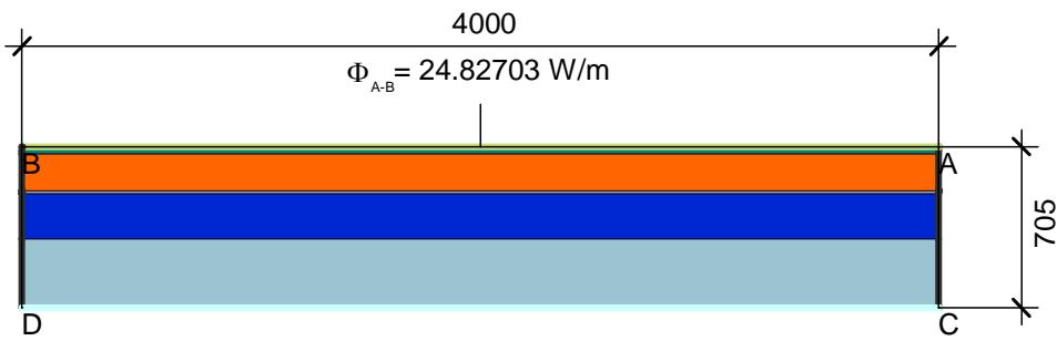
$$U_{eq A-B} = \frac{\Phi}{\Delta T \cdot b} = \frac{24.827}{30.000 \cdot 4.000} = 0.207 \text{ W/(m}^2 \cdot \text{K)}$$
