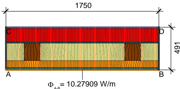
$$U_{\text{eq A-B}} = \frac{\Phi}{\Delta T \cdot b} = \frac{10.279}{30.000 \cdot 1.750} = 0.196 \text{ W}/(\text{m}^2 \cdot \text{K})$$
