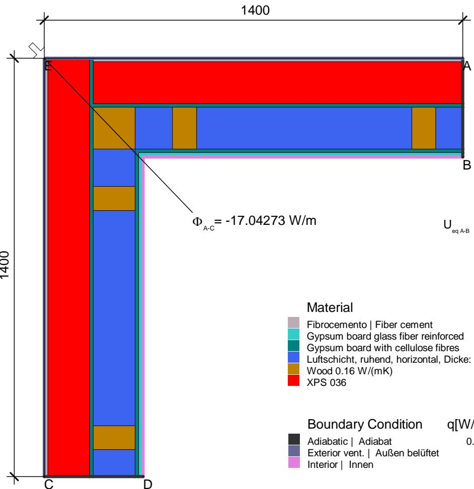
$$\psi_{A-E-C, \cdot} = \frac{\Phi}{\Delta T} - U_1 \cdot b_1 - U_2 \cdot b_2 = \frac{17.043}{30.000} - 0.224 \cdot 1.400 - 0.224 \cdot 1.400 = -0.059 \text{ W/(m}\cdot\text{K)}$$
