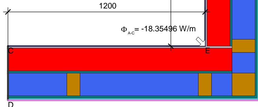
$$\psi_{A-E-C, +} = \frac{\Phi}{\Delta T} - U_1 \cdot b_1 - U_2 \cdot b_2 = \frac{18.355}{30.000} - 0.224 \cdot 1.200 - 0.224 \cdot 1.200 = 0.074 \text{ W/(m} \cdot \text{K)}$$
