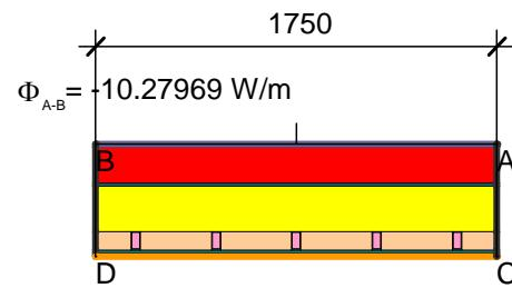
$$U_{eq\ A-B} = \frac{\Phi}{\Delta T \cdot b} = \frac{10.280}{30.000 \cdot 1.750} = 0.196 \text{ W/(m}^2\text{·K)}$$
