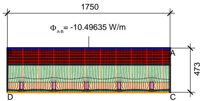
$$U_{\text{eq A-B}} = \frac{\Phi}{\Delta T \cdot b} = \frac{10.496}{30.000 \cdot 1.750} = 0.200 \text{ W}/(\text{m}^2 \cdot \text{K})$$
