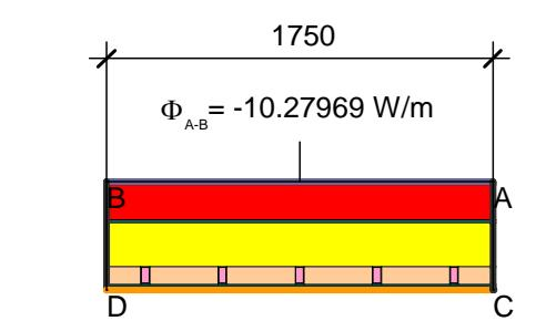
$$U_{eq A-B} = \frac{\Phi}{\Delta T \cdot b} = \frac{10.280}{30.000 \cdot 1.750} = 0.196 \text{ W}/(\text{m}^2 \cdot \text{K})$$
