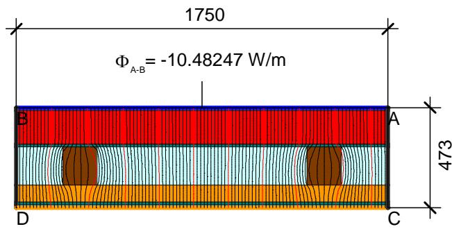
$$U_{\text{eq A-B}} = \frac{\Phi}{\Delta T \cdot b} = \frac{10.482}{30.000 \cdot 1.750} = 0.200 \text{ W}/(\text{m}^2 \cdot \text{K})$$
