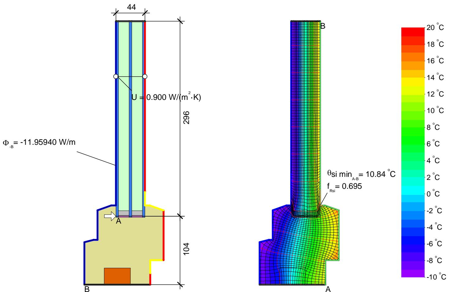
$$\psi_{edA} = \frac{\Phi}{\Delta T} - U_g \cdot b_g - U_f \cdot b_f = \frac{11.959}{30.000} - 0.900 \cdot 0.296 - 1.036 \cdot 0.104 = 0.025 \text{ W}/(\text{m} \cdot \text{K})$$
