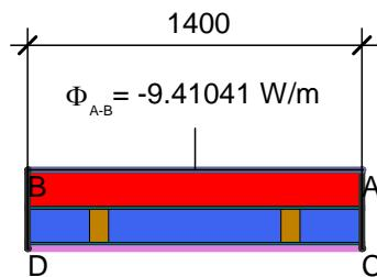
$$U_{eq A-B} = \frac{\Phi}{\Delta T \cdot b} = \frac{9.410}{30.000 \cdot 1.400} = 0.224 \text{ W/(m}^2 \cdot \text{K)}$$
