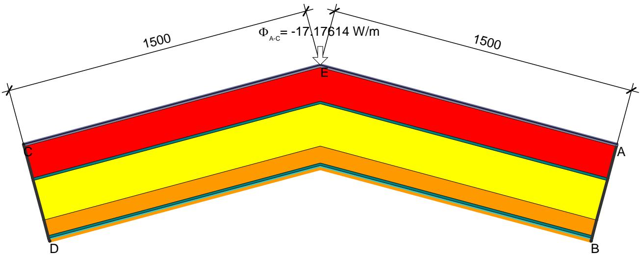
$$\psi_{A-E-C,*} = \frac{\Phi}{\Delta T} - U_1 \cdot b_1 - U_2 \cdot b_2 = \frac{17.176}{30.000} - 0.196 \cdot 1.500 - 0.196 \cdot 1.500 = -0.015 \text{ W/(m}\cdot\text{K)}$$
